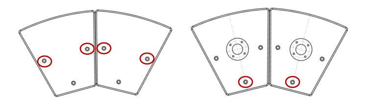
2 Screw the lower hardware link and the fly bar into the indicated points:
